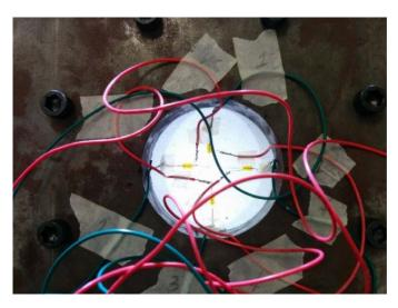
Figure 3. Upper surface of the Mylar sample showing attached strain gages.
